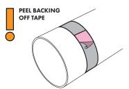
TAPE WIDER THAN ELEMENT RING DOUBLE UP IF REQUIRED
